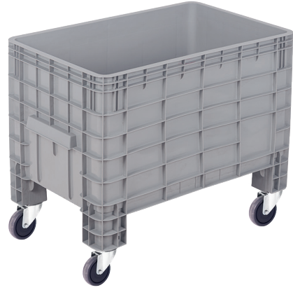
TP-400 T En/W Boy/L Yük/H Hacim Dynamic Static Dış / Ext 636 x 1017 x 790 mm Volume Capacity Capacity İç / Int 585 x 932 x 512 mm 270 Lt 300 Kg 1800 Kg Kapalı / Closed Ağırlık / Weight 14,50 kg
